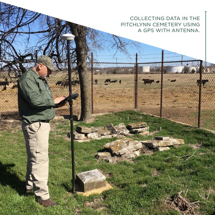
COLLECTING DATA IN THE PITCHLYNN CEMETERY USING A GPS WITH ANTENNA.
